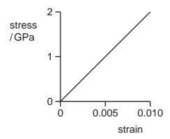
What is the strain energy per unit volume of a rod made from this metal when the strain of the rod is 0.010?
