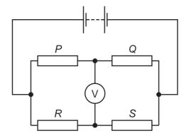
The voltmeter reading is zero.
